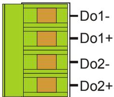
2 pulse / state digital outputs are available on the device.
