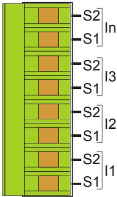
**Current measurements** can be performed by connecting the terminals of Current inputs.
