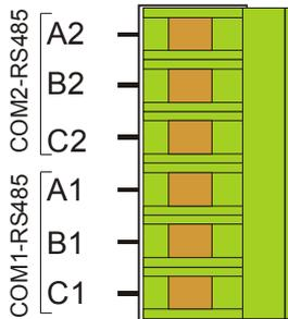
Depending on the version, the instrument can be equipped with one or two isolated half duplex RS485 serial interface.
