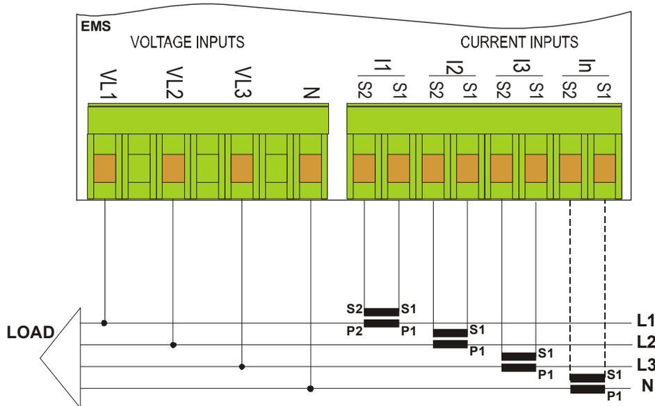
In case of connection in a 3 phase network (without neutral or with neutral not distributed) don't connect the N terminal.
