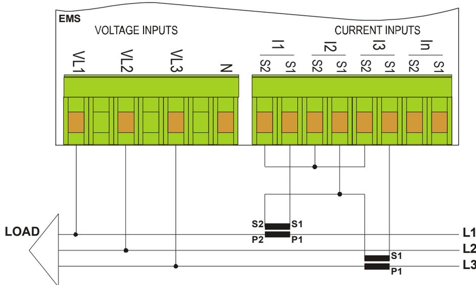
This connection with only 2 CT allows to measure accurately the three-phase currents.
