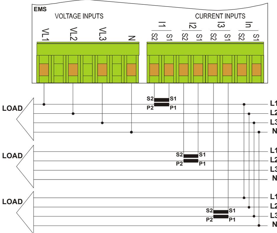
In presence of multiple balanced loads in a three-phase network, the instrument calculates the electrical parameters checking a single phase current for each load, allowing to limit the number of CT used.
