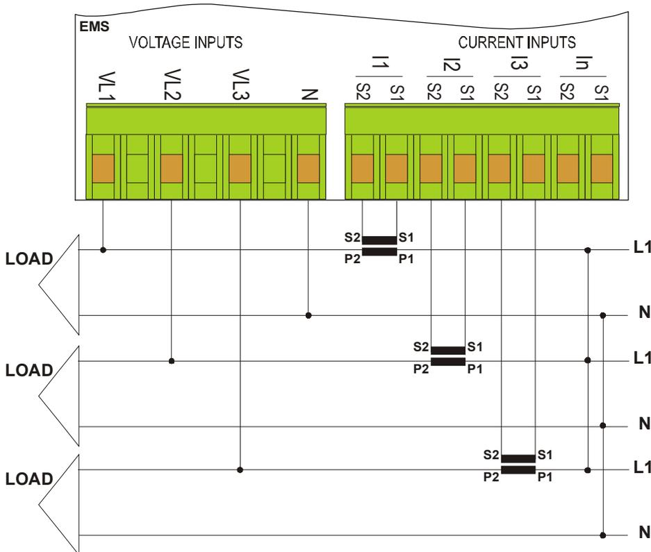
The electrical parameters are measured for individual loads. For correct calculation of power and energy, is mandatory to connect the voltage inputs related to the used current inputs.
