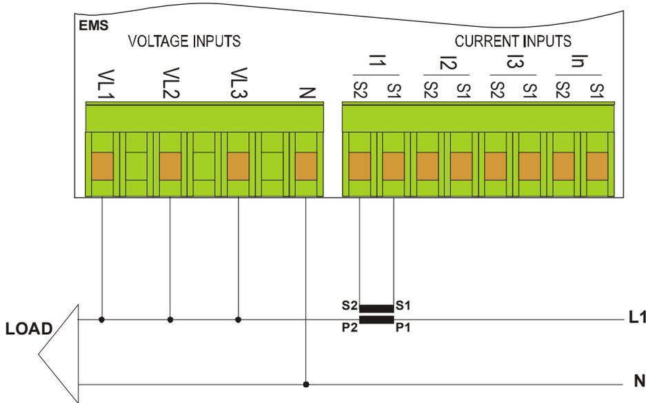
It is mandatory to connect the current input I1 and voltage input VL1.
