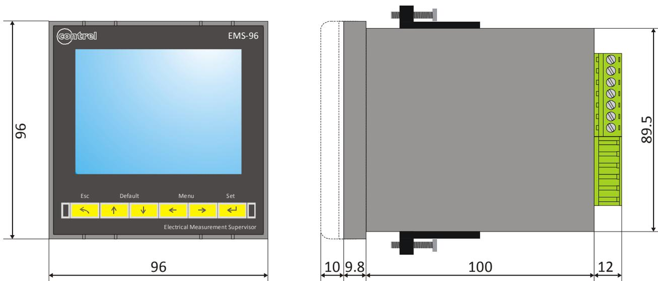
For fixing the flush mount version instrument to the panel, use the fixing devices supplied, by inserting them in the side grooves of the enclosure and tighten the screws.
