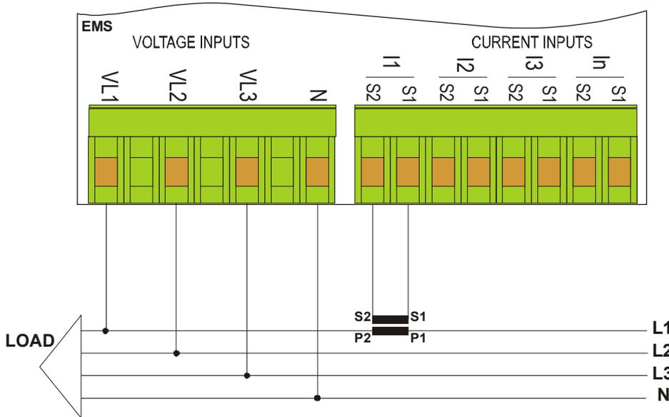
This connection can be used with distributed and equal loads.
