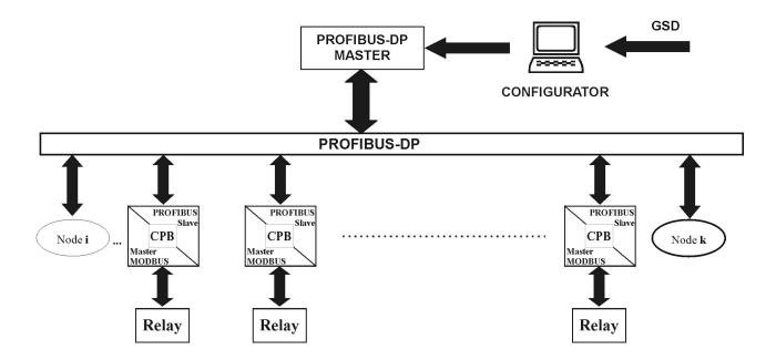
Fig. 1: Block scheme of the measuring system with the CPB converter.
