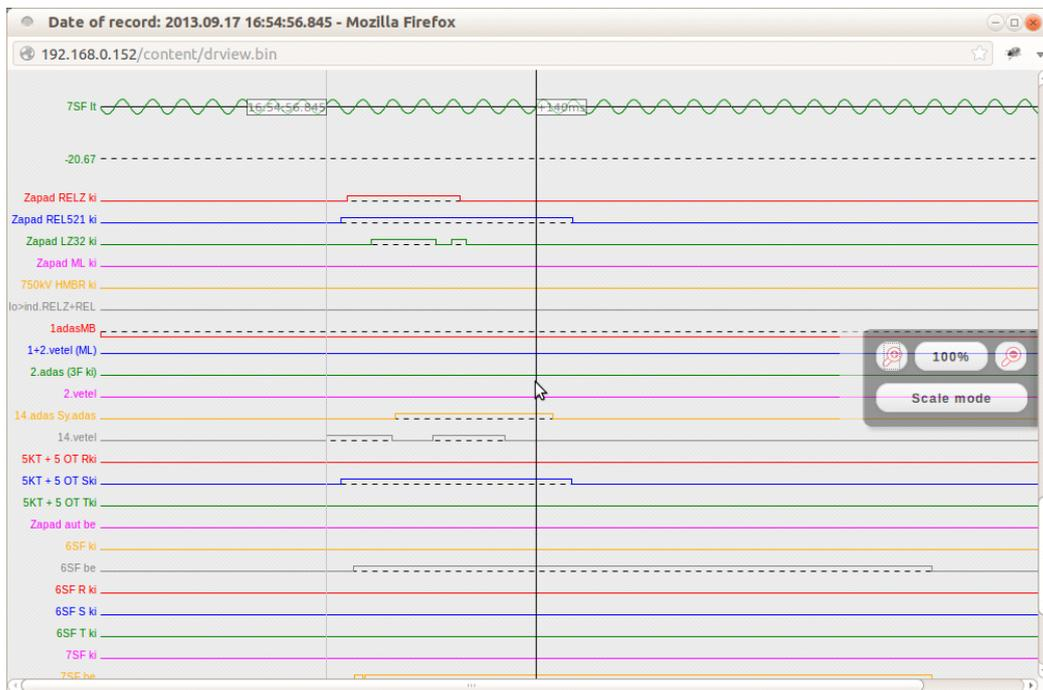
Fig.10. Disturbance record's binary channels
