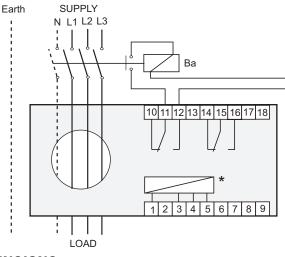
Wiring diagram with shunt trip of the MCCB and excited end relay (N) for fail safe (F.S.) Connect terminals 10-11 to BA (NO contact under non tripped condition)
