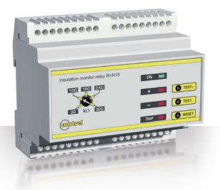
The RI-R15 device allows the permanent insulation monitoring to earth of electric networks in direct current isolated (IT systems). Insulation resistance monitoring is carried out measuring the potential variation of two polarity on ground reference. Auxiliary supply is taken from under-control network.
