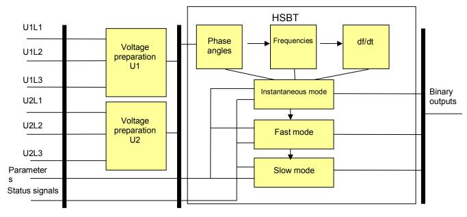
Figure 1-2 shows the structure of the high speed bus transfer function (HSBT).
