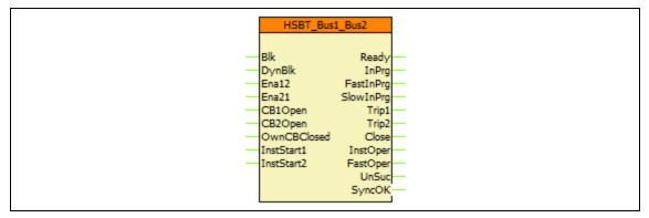
Figure 1.4-1 The function block of the high speed bus transfer protection function
