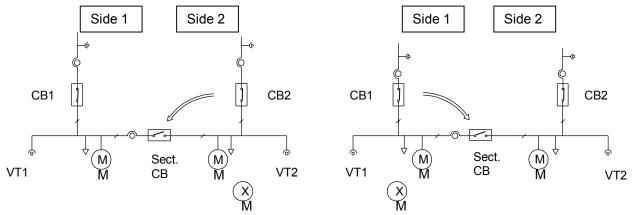
Figure 1-1 Simple switchgear configuration
