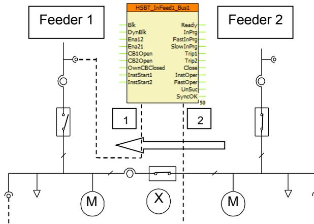
*Figure 2-4 Application of the HSBT Infeed1-Bus1 instance*
