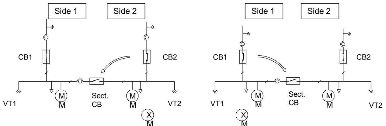
Figure 1-1 Simple switchgear configuration
