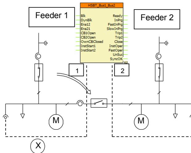
*Figure 2-2 Application of the HSBT Bus1-Bus2 instance /1*
