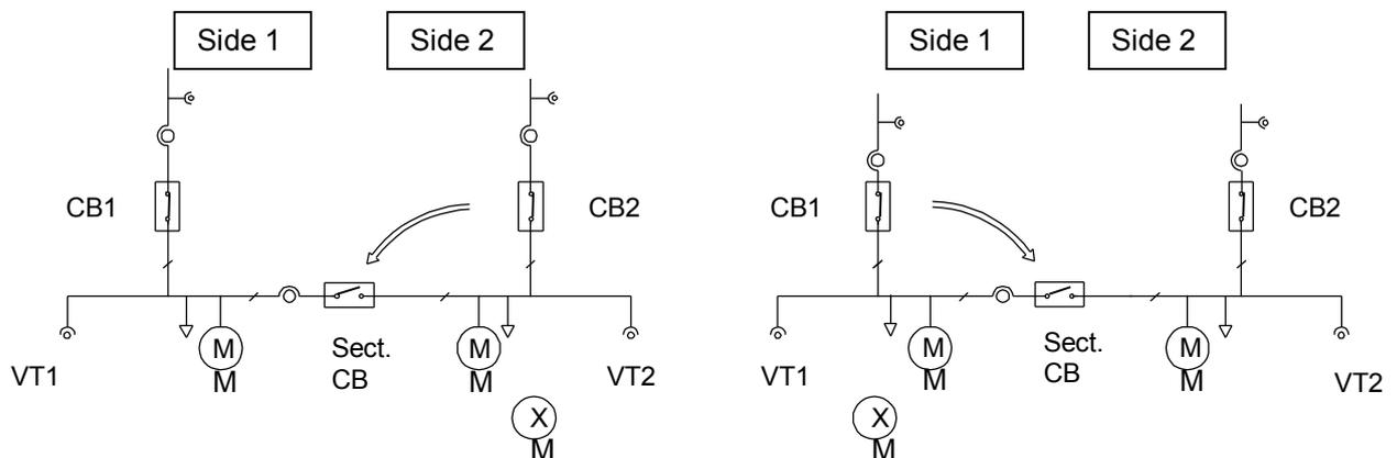
Figure 1-1 Simple switchgear configuration
