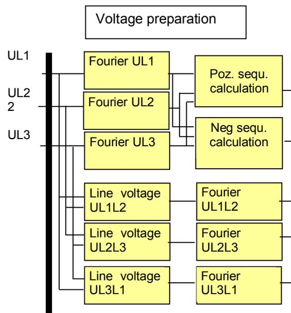
*Figure 1-3 Structure of the voltage preparation algorithm*
