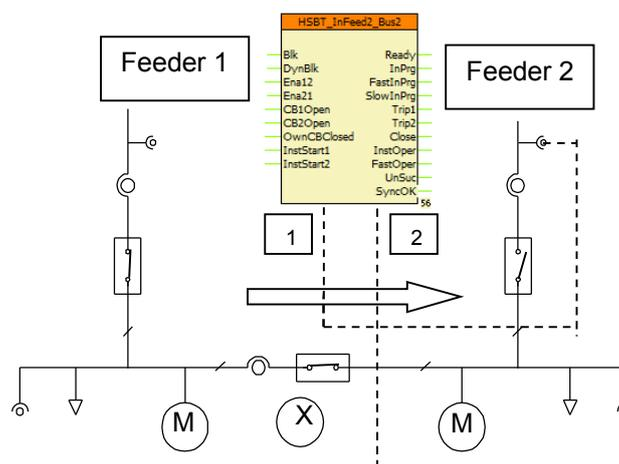
*Figure 2-5 Application of the HSBT Infeed2-Bus2 instance*
