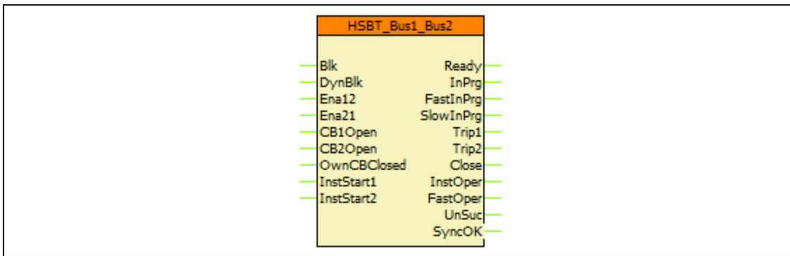
Figure 1.4-1 The function block of the high speed bus transfer protection function
