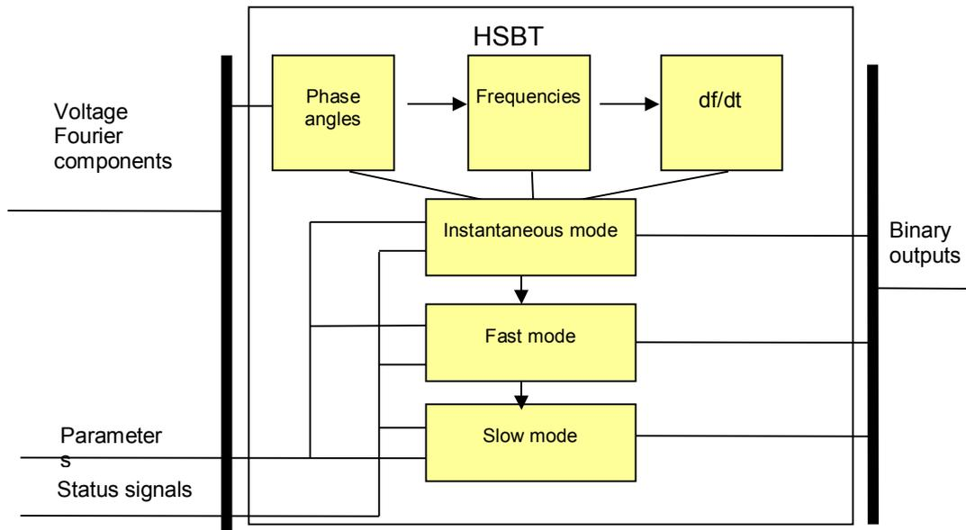
Figure 1-4 Principal structure of the HSBT algorithm
