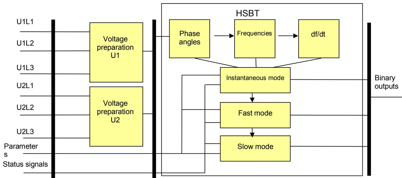
Figure 1-2 Structure of the high speed bus transfer function
